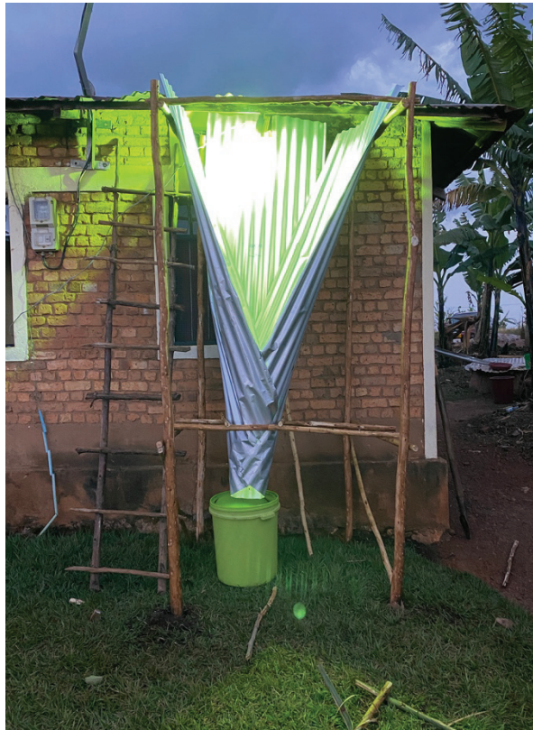
A "traditional" senene trap adapted to collect moths and coleoptera (Kagera, Karagwe district)
