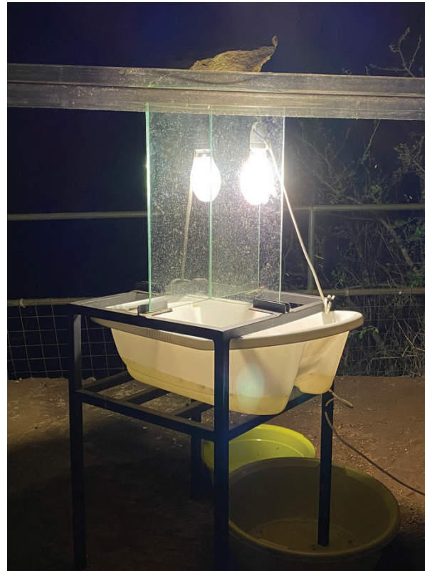
A "modern" light trap with windows and mercury lamp
